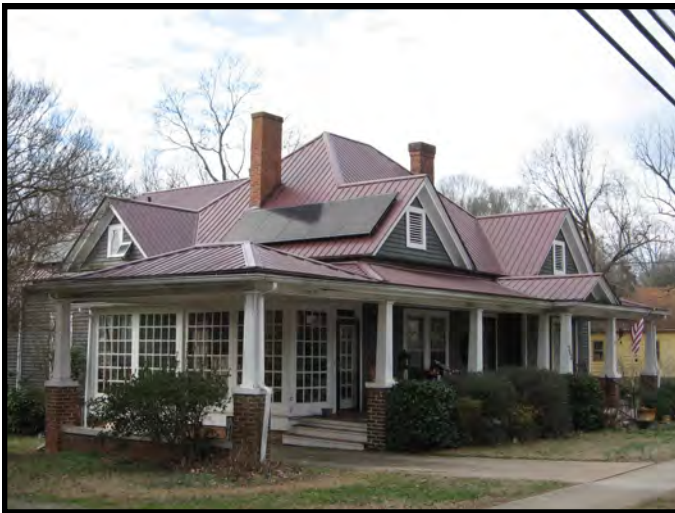
NO —Solar panels should not be placed on primary facades or readily visible locations.
