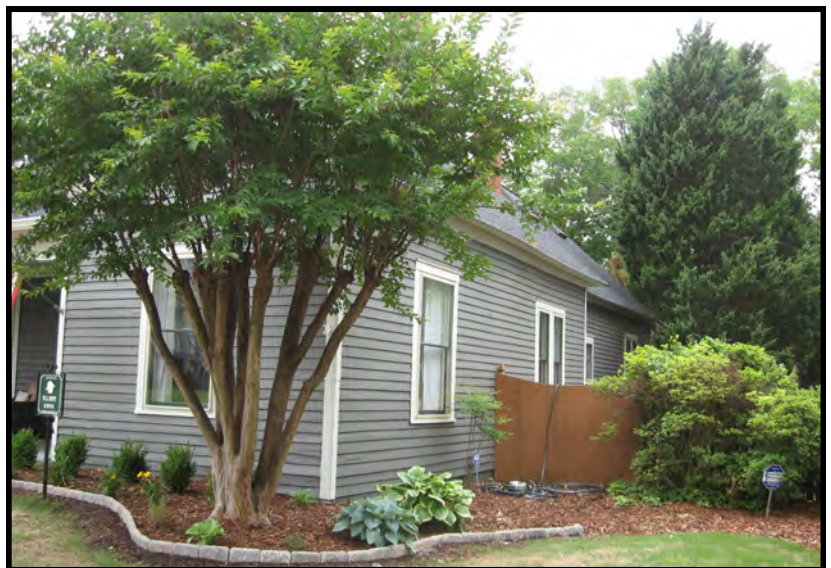
Privacy fences to enclose rear yards are appropriate and should be at least halfway back from the front wall of the house as at 113 Cain Street, NE.
