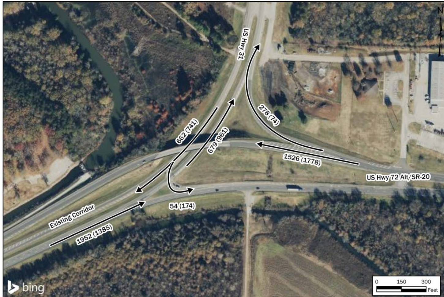
Figure 1.3.3.1-2. Existing Peak Hour Volume for U.S. Highway 31 and U.S. Highway 72 Alt/SR-20 Interchange (AM/PM)
