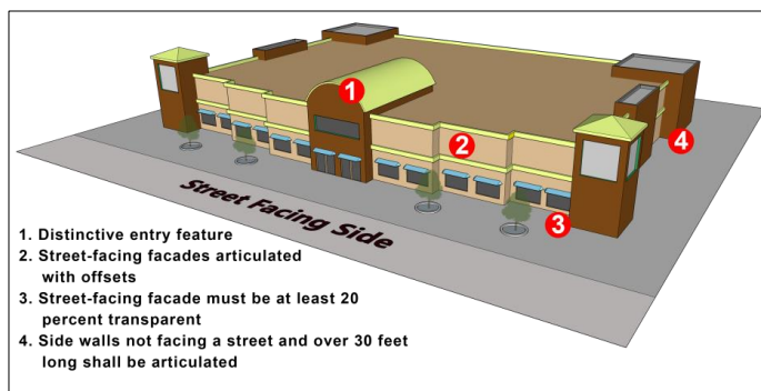
Figure 25-5.7.5(b)(2): Large Retail Building Entrances and Massing
